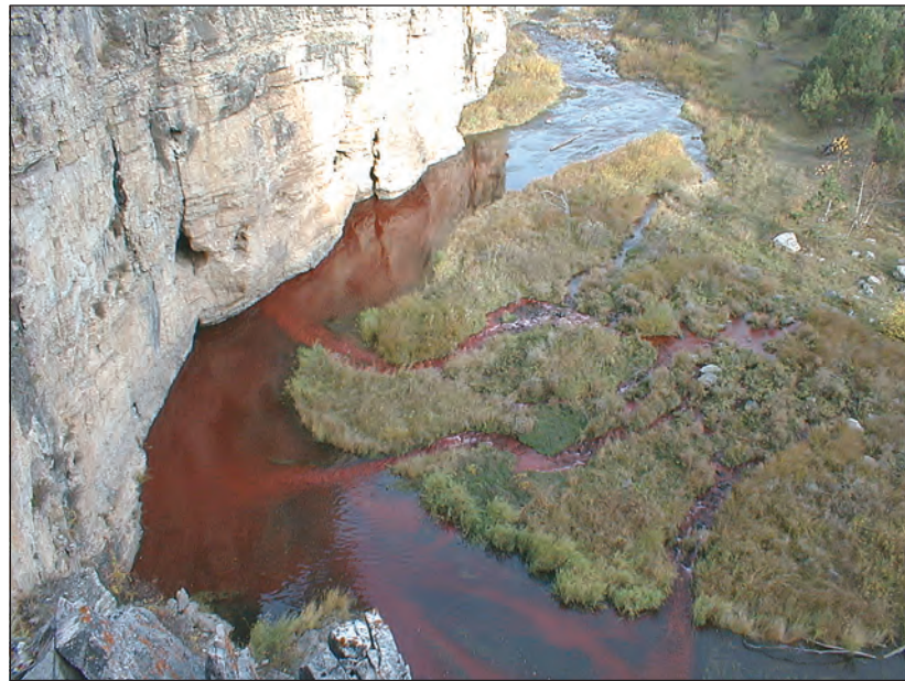
Figure 18. Example of the use of dye to examine water fluxes between surface water and ground water (from Carter and others, 2002). Dye testing has been done in Boxelder Creek, South Dakota, which can lose as much as 50 cubic feet per second of flow to the bedrock aquifers. In the upper left photograph, nontoxic, red dye is poured into Boxelder Creek upstream from a major loss zone. In the upper right photograph, dye in the stream can be seen disappearing into a sinkhole in the Madison Limestone. In the bottom photograph, dye in the stream emerges downstream at Gravel Spring, which is about 671 meters (2,200 feet) (linear distance) from the major loss zone. The length of time for the first arrival of dye to travel this distance is variable depending on flow conditions but generally is about 1 to 2 hours (Strobel and others, 2000). Thus, the ground-water velocity is about 0.3 to 0.6 kilometer per hour (0.2 to 0.4 mile per hour), which is a very fast rate for ground water. Dye also has been recovered at City Springs, which is in the Rapid Creek Basin, about 30 days after injection. This demonstrates that ground-water flow paths are not necessarily restricted by surface-water drainage basins. (Photographs by Derric L. Isles, South Dakota Department of Environment and Natural Resources.)
