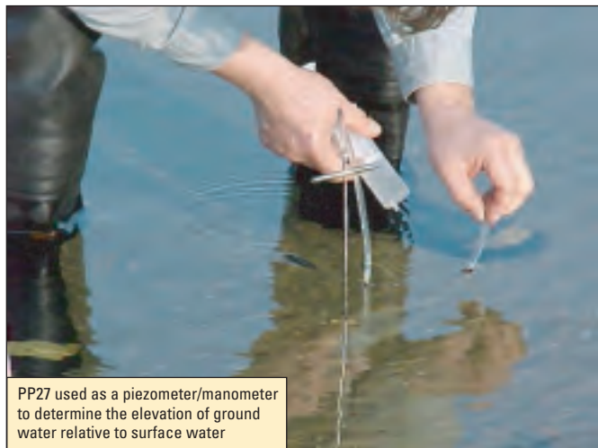
Figure 12. MHE PP27 probe used to indicate difference in head (modified from Henry, 2000). (Photograph by Mark Henry, Michigan Department of Environmental Quality.)
