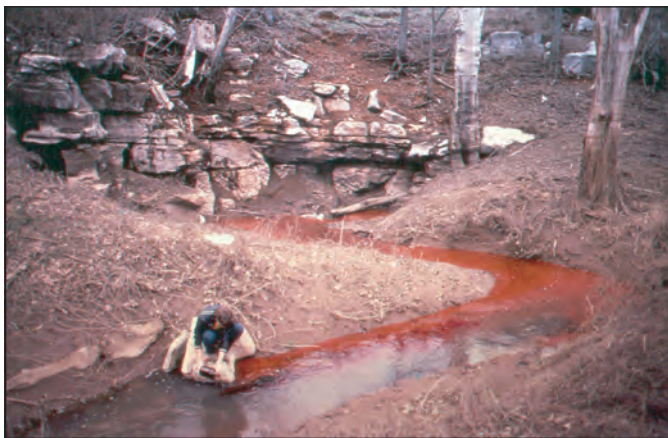
Figure 16. Dye injections: A , sodium fluorescein injection into collapse sinkhole formed in a pond (stream of water is outflow from a settling pond at a public supply water-treatment plant); B , Rhodamine WT injected into sinking stream; C , injection of Rhodamine WT into a water-level observation well (photographs by Charles J. Taylor, U.S. Geological Survey).
