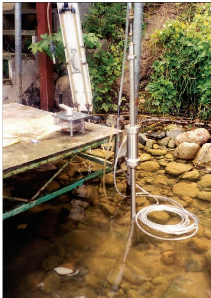
Figure 8. Hydraulic potentiometer probe with drive hammer shown driven about 2 meters beneath the lakebed. Manometer and hand-crank peristaltic pump are visible in background. (Photograph by Donald Rosenberry, U.S. Geological Survey.)
