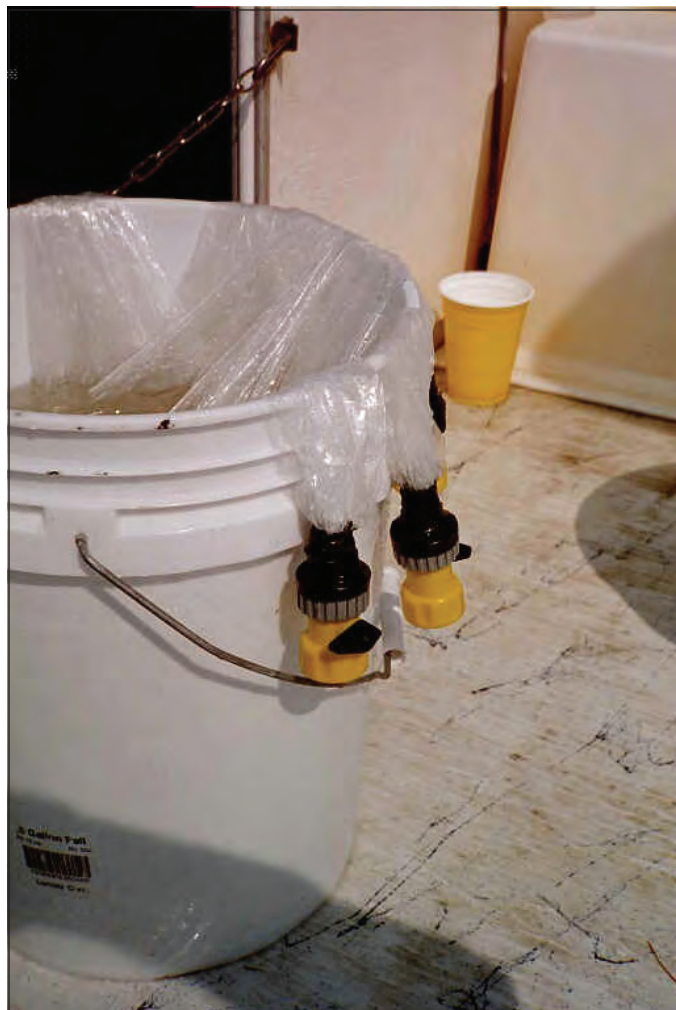
Figure 16. Plastic bag attached to a garden-hose shut-off valve. Bag is filled with a known volume of water and then purged of air. Valve is closed. Bag is threaded onto male threads on seepage meter, and valve then is opened to begin seepage measurement. (Photograph by Donald Rosenberry, U.S. Geological Survey.)
