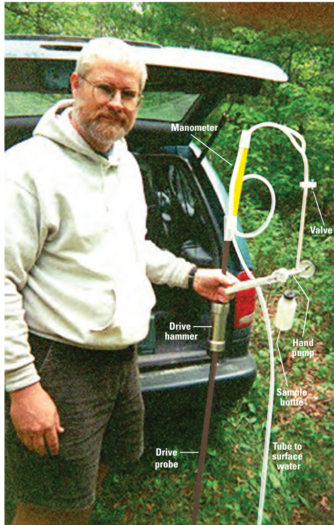
Figure 9. Hydraulic potentiomanometer (created by Joe Magner, Minnesota Pollution Control Agency) with manometer connected to drive probe. Note the proximity of the lake and drive-point tubes to minimize out-of-level errors. Note also the in-line water bottle to keep the vacuum pump dry. (Photograph by Donald Rosenberry, U.S. Geological Survey.)
